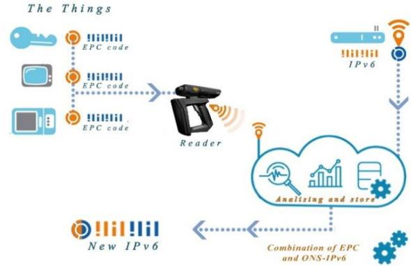
Figure. 3. Combination of EPC with ONS IPv6
